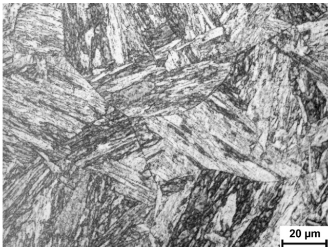
Fig. 4. Optical micrograph showing the grain structure of the EM10 (CEA) steel.
