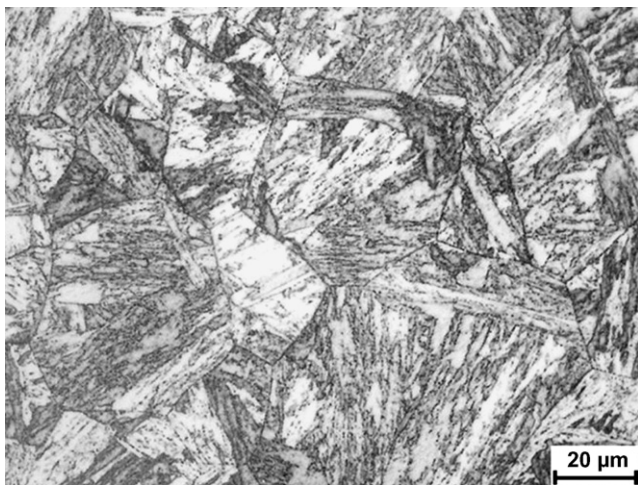
Fig. 13. Optical micrograph showing the grain structure of the Optifer-IX steel.
